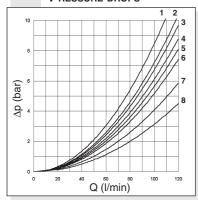
The diagram at the side shows the pressure drop curves for spools during normal usage. The fluid used is a mineral oil with a viscosity of 46 mm²/s at 40°C; the tests have been carried out at a fluid temperature of 40°C. For higher flow rates than those in the diagram, the losses will be those expressed by the following formula:
