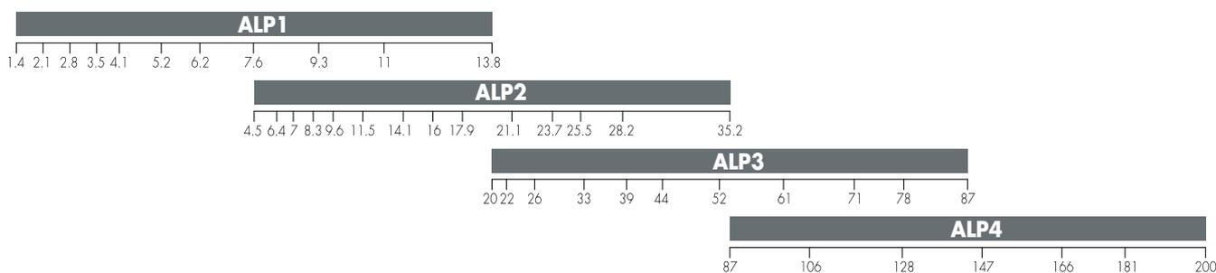
cilindrata [cm<sup>3</sup>/giro] - displacement [cm<sup>3</sup>/rev]
