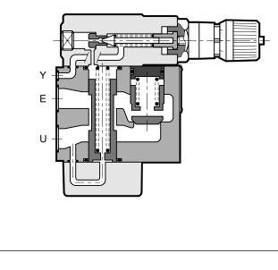
The Z\*-P type valves are used when a branch with a lower pressure than the main one is desired in the hydraulic circuits.
